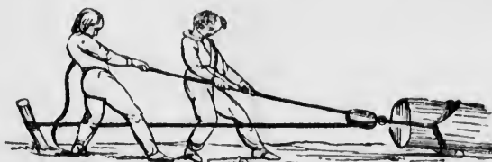
Fig. 305.—APPLICATION OF THE PULLEY.
